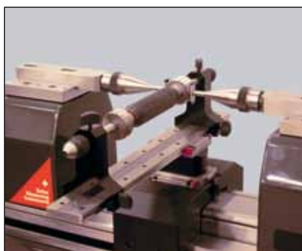
Checking of thread plug gauges (HPA-1/TEL6/3P/0.17-3.2/S6.5/LABC-15)
