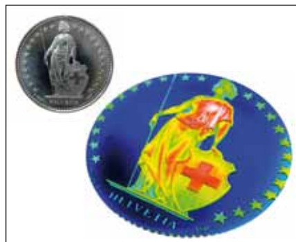
Measurement of macroscopic surface textures (CCM P1)
