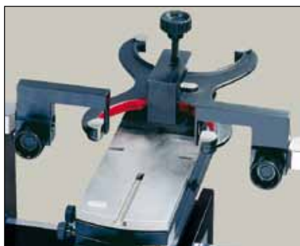
Checking of snap gauges (TA-SU-313/TEL14N)
