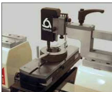
Calibration of thread ring gauges (TA-SU-313/LABC-70/TA-SU-354)
