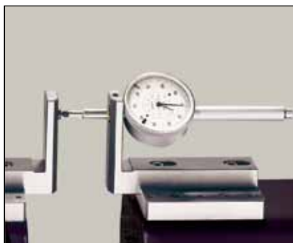
Checking of dial indicators (TEL5CN)
