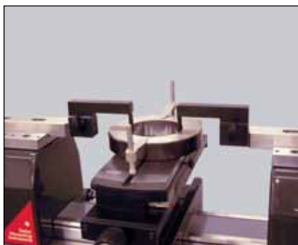
Checking of ring gauges (TA-SU-313/TEL16.1/HPA-1)
