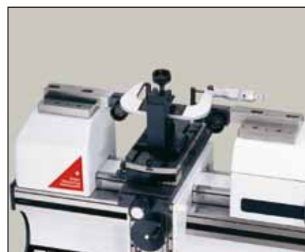
Calibration of external micrometers (HPA-1/TULM14)
