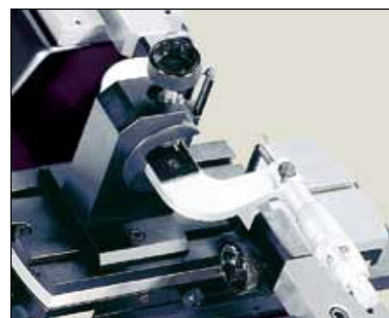
Checking of external micrometers (HPA-1/TULM14)
