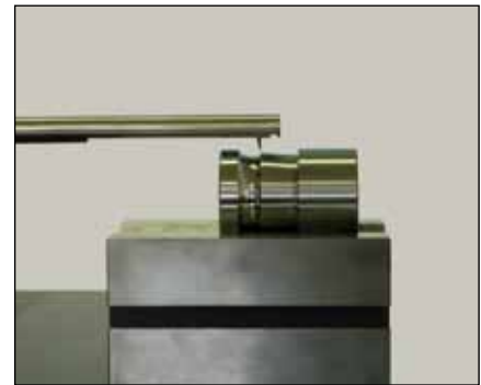
Contour measurement with TR Profile DH-8/VHF (TA-MS-650)
