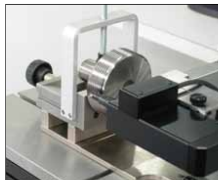
Checking of taper thread plug gauges (TA-MS-381/TEL75)
