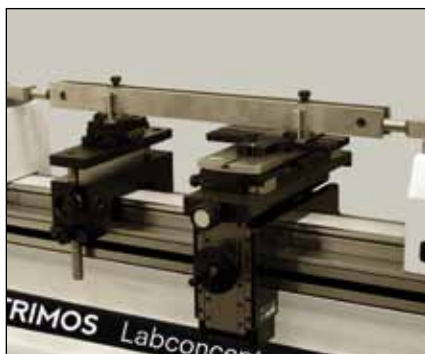
Comparative checking of gauge blocks > 250 mm (TA-SU-313/TELMA7/P/TA- SU-305/TA-SU-306)
