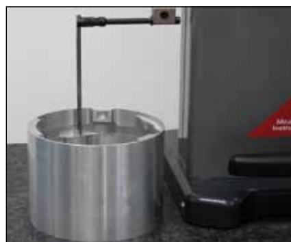
Depth measurement (TA-IH-109/V-50.5/V-50.4)
