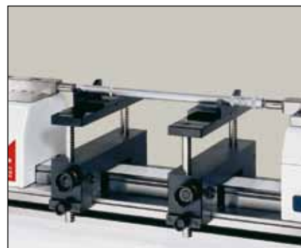
Setting of 2-point internal micrometers (HPA-1/TELMA7/TELMN7.2)
