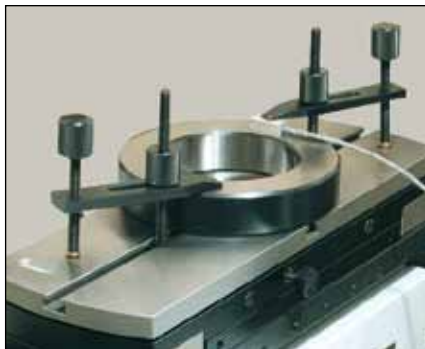
Integrated temperature compensation system TempComp
