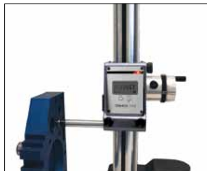
Measuring of centerline distances (TVM5)
