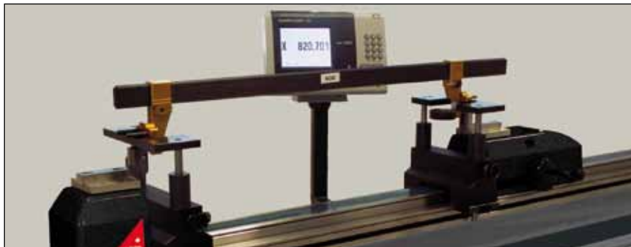
Setting of a large gauge (TEL5)
