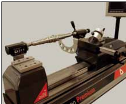
HPA: Measurement of cylindrical parts (TA-MS-303)
