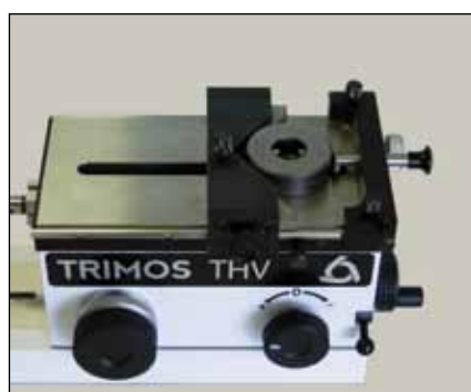
Calibration of plain rings gauges (THV-260)
