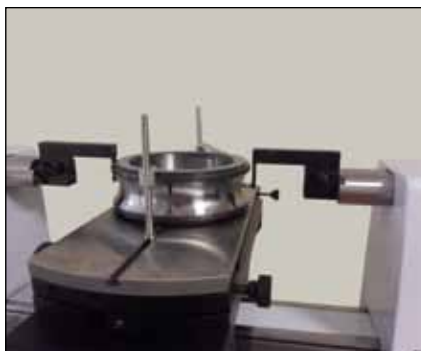
CNC controlled external measurement of a bearing ring
