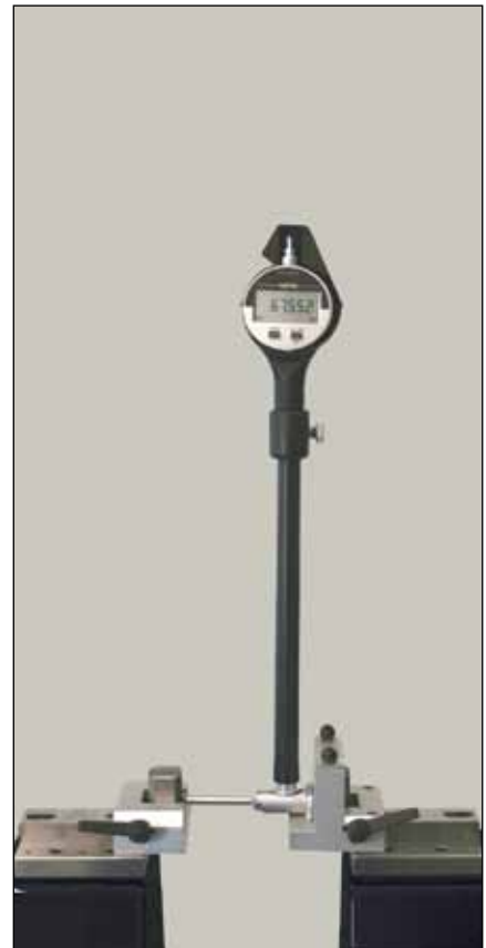
Setting of 2-point bore gauges (TEL5/TA-SU-301)
