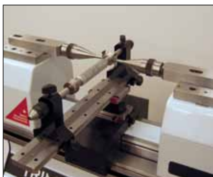
Calibration of thread plug gauges (HPA-1/TEL6/3P/0.17- 3.2/S6.5/LABC-15)
