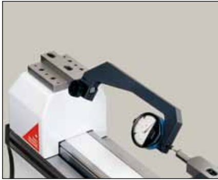
Checking of dial indicators (TULM5C)
