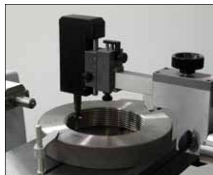
Calibration of thread ring gauges (TA-MS-370/TEL75/TA-SU-354)
