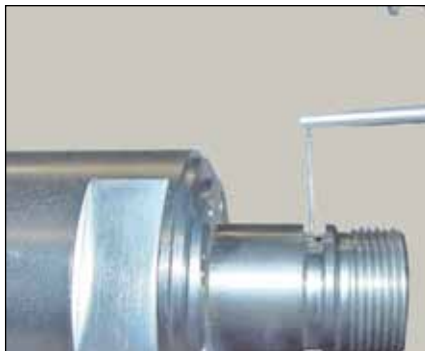
Checking at recessed measuring points (TA-MS-609)
