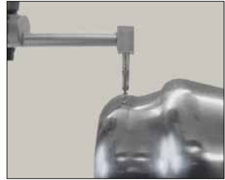
Measuring surface roughness of a polished part (TA-MS-607)
