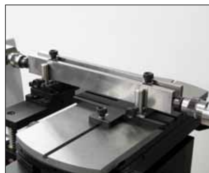
Comparative checking of gauge blocks > 250 mm (TA-SU-307/TEL7/TELMA7)
