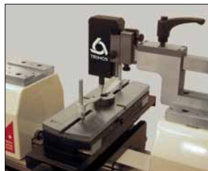
Calibration of small ring gauges (TA-SU-313/LABC-70/TA-SU-354)
